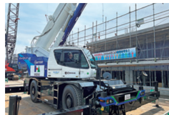
Adoption of battery-powered full-electrified rough terrain cranes
