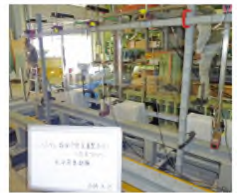
Handrail horizontal load test
