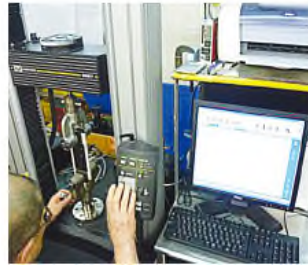
Test to confirm performance of waterproofing material
