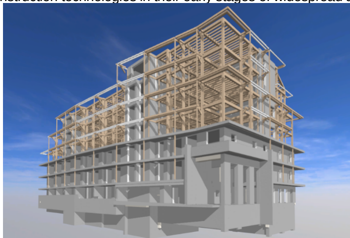
Model diagram of wood and reinforced concrete hybrid structure
