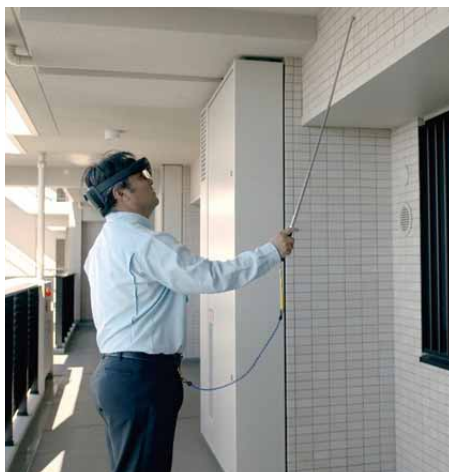
Hammering test conducted by wearing HoloLens2
