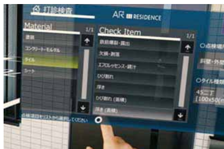
Screen of inspection record item selection
