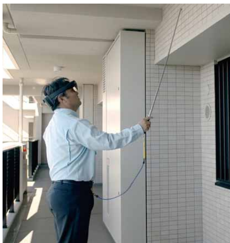
Hammering test conducted by wearing HoloLens2
