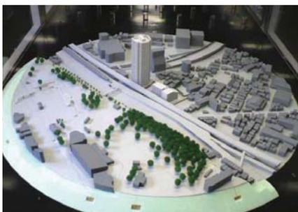
Wind tunnel tests
