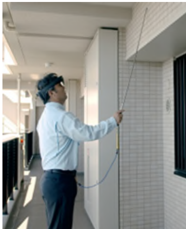
Hammering test conducted by wearing HoloLens2
